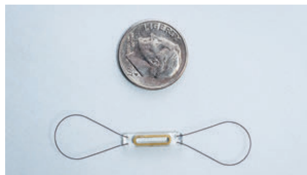
The CardioMEMS™ device is an implanted sensor that checks for increased pressure in the pulmonary artery.
